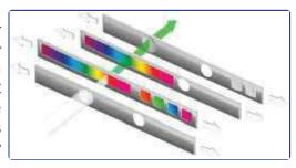
The ATL contains two LVF Monochromators, one for excitation and one for emission. In addition, a Linear Variable Dichroic mirror (340 - 740 nm) separates the two LVF Monochromators.
